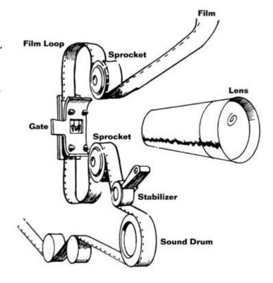
eliminate the inevitable difference in apparent sharpness at the point of projection and actual sharpness at the surface of the screen. Where academy leader is provided, use the leader for fine pre-focusing, then lock and do not attempt to refocus for the remainder of the reel.
